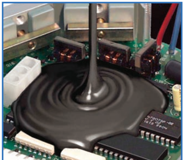
Potted electronics make imPulse highly reliable, even in damp locations.
